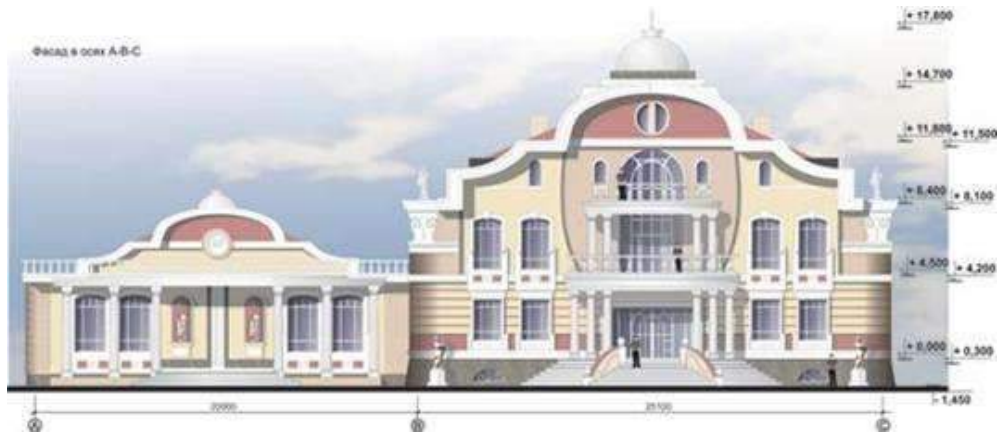
Figure 6.5 - Drawing of the building facade
